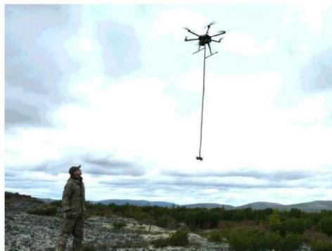
Figure 1. “Heavyweight” multirotor with magnetometer in flight.
