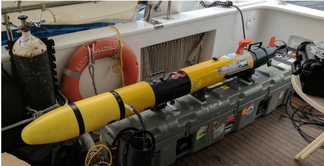
**Figure 1.** Sensor system in long housing attached to REMUS 100 autonomous underwater vehicle
